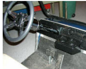
Step 6: Attach the U-Joint to the column and retighten the U-Joint bolt and the column support bolts.
