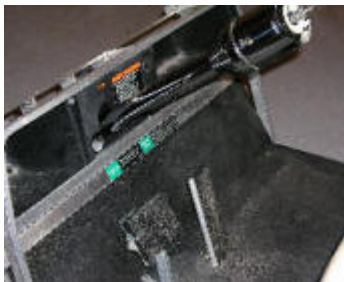
Step 5: Slide the column into the lower column support. Wires should exit the column at 12 o'clock.
